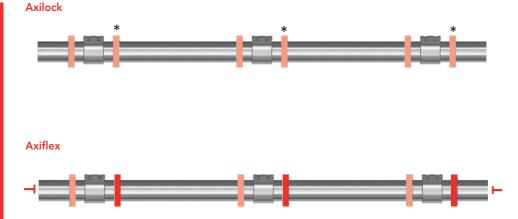
Axiflex pipe couplings are not designed to accept end load pressures. As a result, pipes must generally be anchored against internal pressure at changes in direction, branches, valves and at pipe ends and secured by fixed points and guides.
